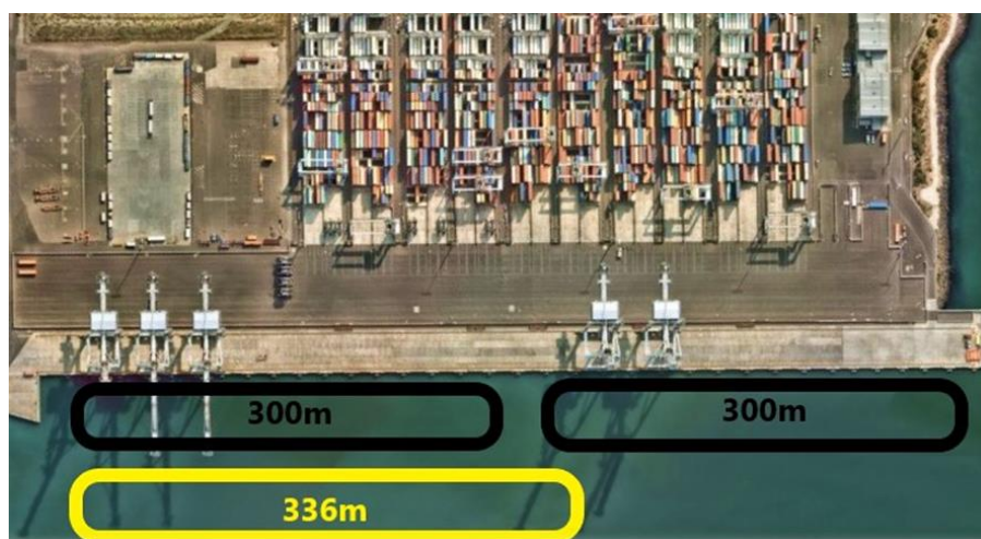
Figure 18: WDE overview with 300m design vessels vs actual 336m vessels resulting in the terminal becoming a one berth terminal
