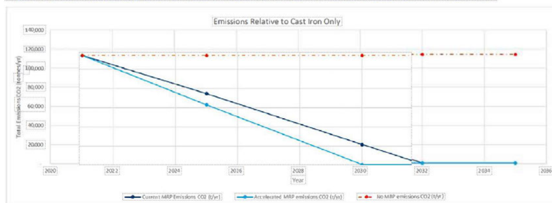
Figure 1: Estimated fugitive emissions reductions as a result of cast iron MRP for MGN
